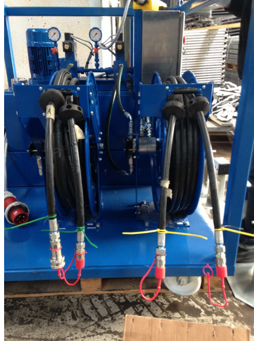
Bespoke HPU with a small pump set and hose reels.
